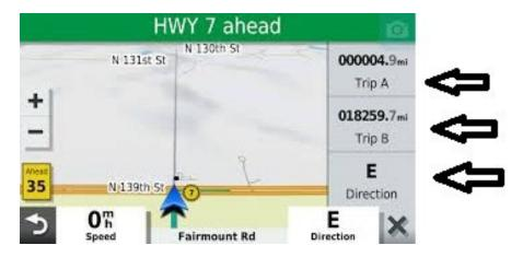
The screen above shows the normal display with Trip Data added (three arrows). You can select whatever data elements you wish to display in the side bar and in what order. Of course you will want to keep TRIP B visible. You can hide the side bar by clicking on the X in the lower right corner. (Note this is not an exact replica of a DriveSmart 76 screen, but was the closest I could find.)
