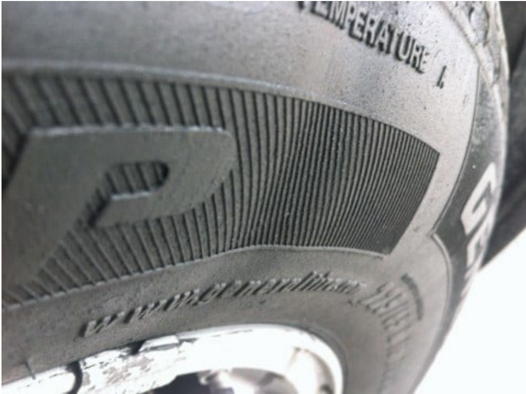
Normal belt overlap depression on a radial tire
